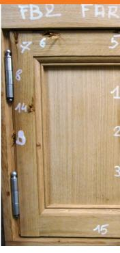
THE BANC NATIONAL D'EPREUVE PERFORMS BALLISTIC RESISTANCE TESTING ON CONSTRUCTION PRODUCTS
