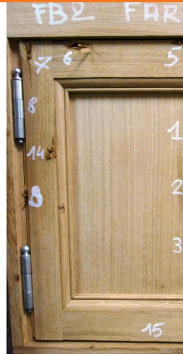
THE BANC NATIONAL D'EPREUVE PERFORMS BALLISTIC RESISTANCE TESTING ON CONSTRUCTION PRODUCTS
